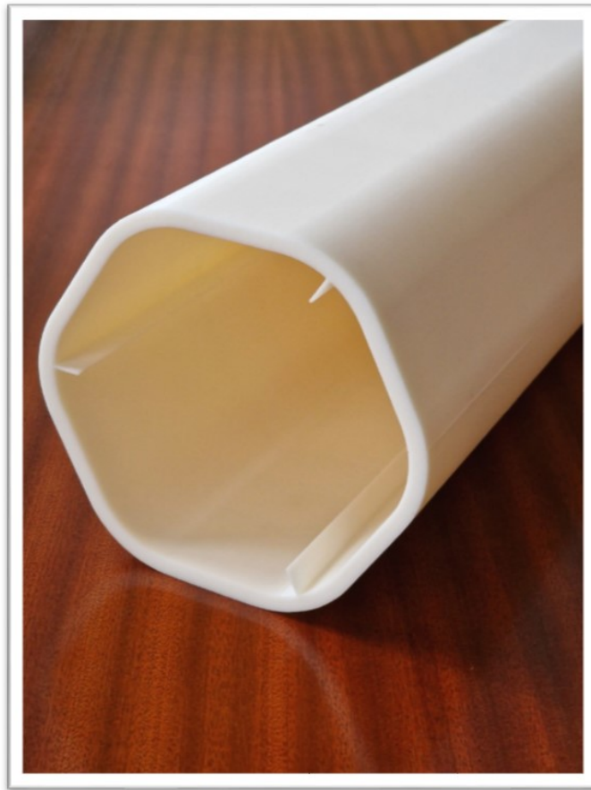
Figure 2. The pipe with the cross-section determined by the range set RS_{\mathcal{F}}(\{0\}) .
